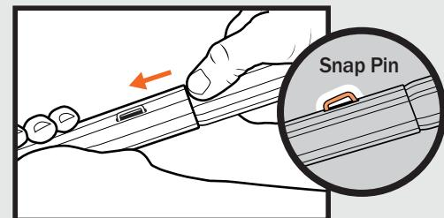
\*To disassemble, push snap pin down & pull.
