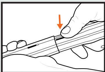
**2** Align top section of poles until snap pin engages in hole.
