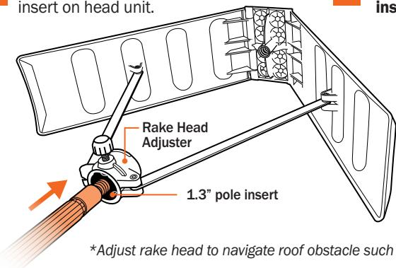
**2** While keeping the holes aligned, insert **TOP** pole into head unit.
