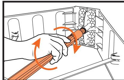
\*Adjust rake head to navigate roof obstacle such as roof vents, pipe jacks, turtle vents and valleys.
