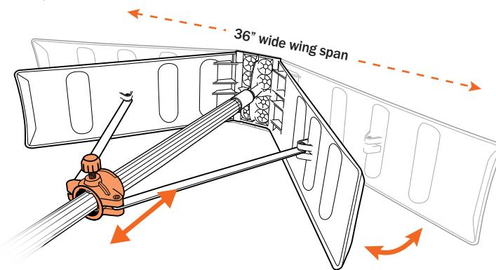
**5** Hand-tighten\* Rake head adjuster **knob** to secure rake position.
