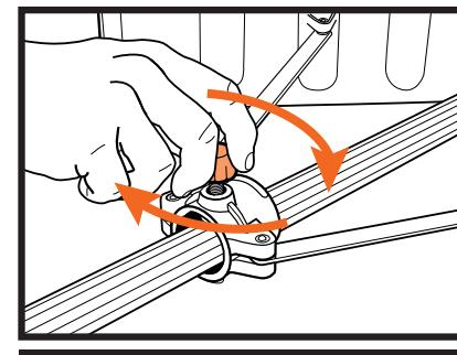
**DO NOT USE PLIERS OR OVER-TIGHTEN THE THUMB SCREW**
